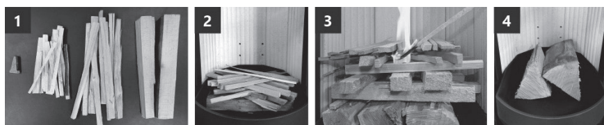
Fig. 4 Placements of wood in the chamber
